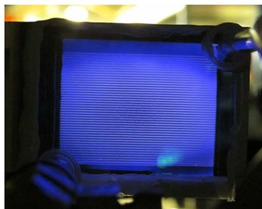
Figure 10. Microplasma reactor for ozone generation: Cutaway view and a 48-channel planar array of Al/Al 2 O 3 microchannels.
